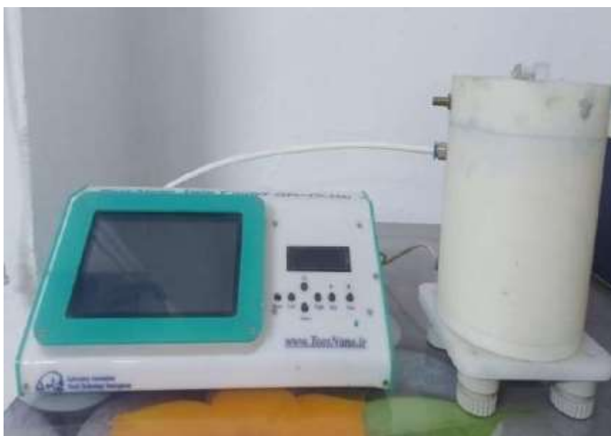
Figure 01- In the present experiment, a spin coating apparatus was used.
